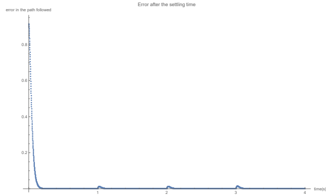
Figure 7.7: Error in the followed vs desired rectangular path by SRSPM
