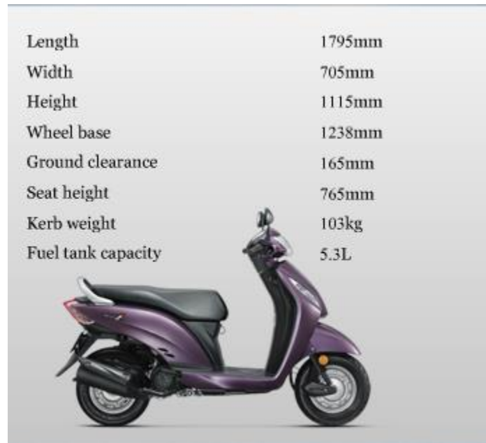
Fig. Activa and its dimensions
